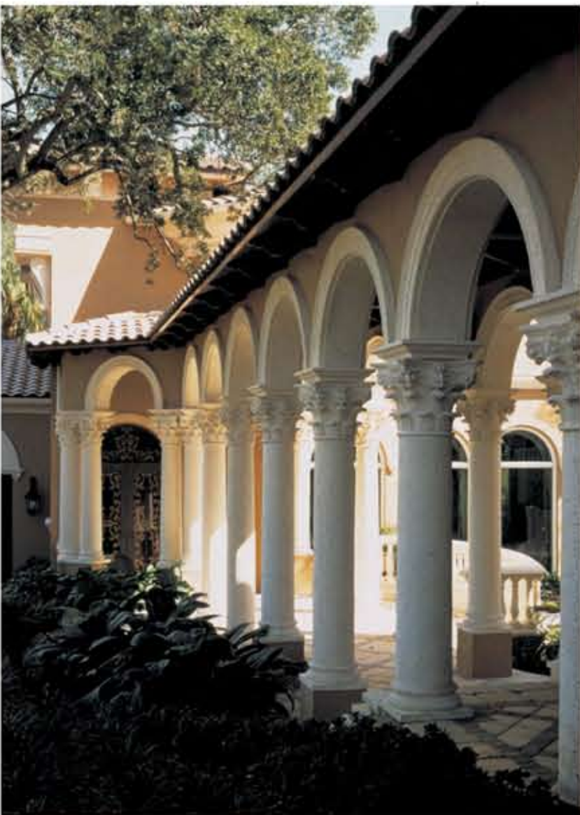
Loggias provide natural cooling with shade and also by blocking direct sun rays from entering the house.
